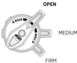
The **3-Position Micro Adjust** lever is useful to make on-the-fly adjustments to control fork performance. Use the positions between the OPEN, MEDIUM, and FIRM modes to fine-tune your compression damping.
