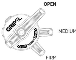
The **3-position lever** is useful to make on-the-fly adjustments to control fork performance under significant changes in terrain, and is intended to be adjusted throughout the ride.
